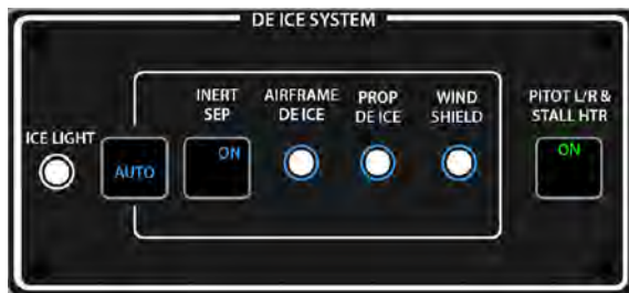
Figure 7.14.2 - DE ICE SYSTEM panel - AUTO mode with ice detected
