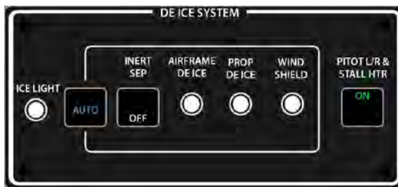
Figure 7.14.1 - DE ICE SYSTEM panel - AUTO mode with no ice detected
