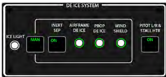
Figure 7.14.3 - DE ICE SYSTEM panel - MAN mode activated
