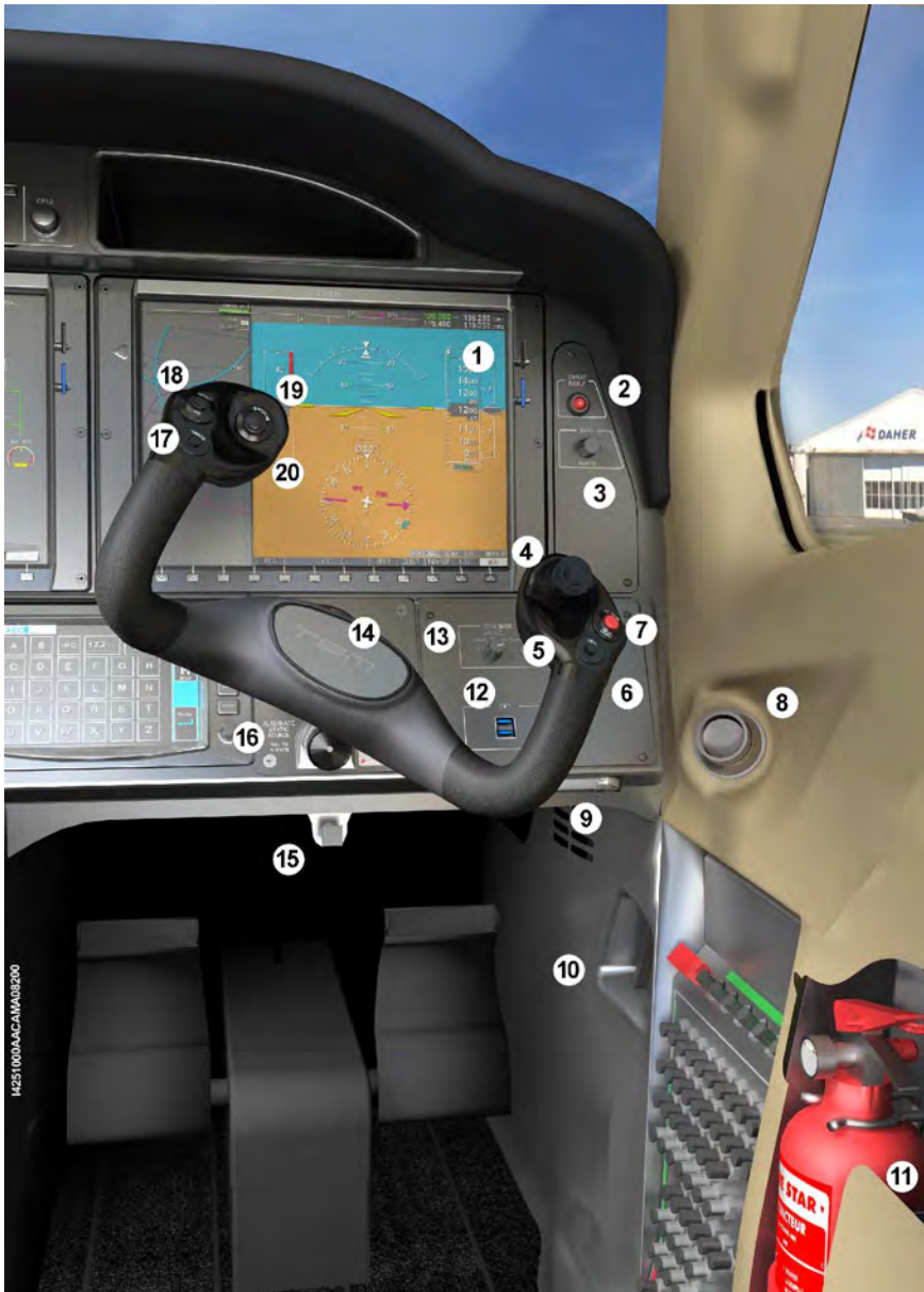
Figure 7.3.5 (2/2) - Right instrument panel (Typical arrangement)
