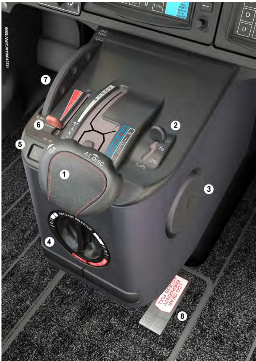
Figure 7.3.6 (2/2) - Pedestal console (Typical arrangement)
