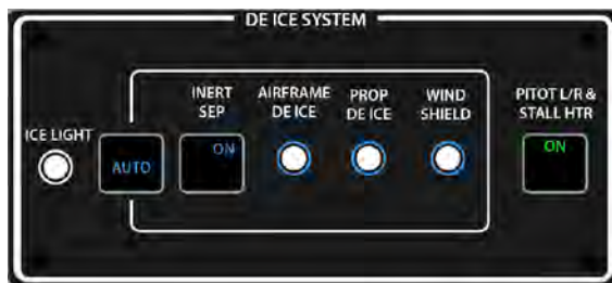
Figure 7.13.2 - DE ICE SYSTEM panel - AUTO mode with ice detected
