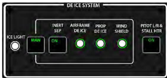
Figure 7.13.3 - DE ICE SYSTEM panel - MAN mode activated
