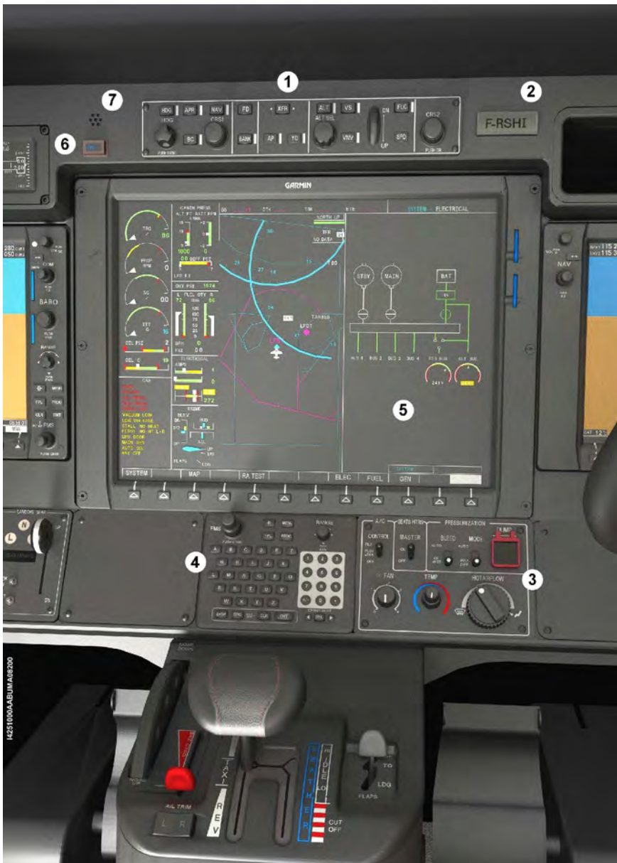
Figure 7.3.4 (2/2) - Central instrument panel (Typical arrangement)
