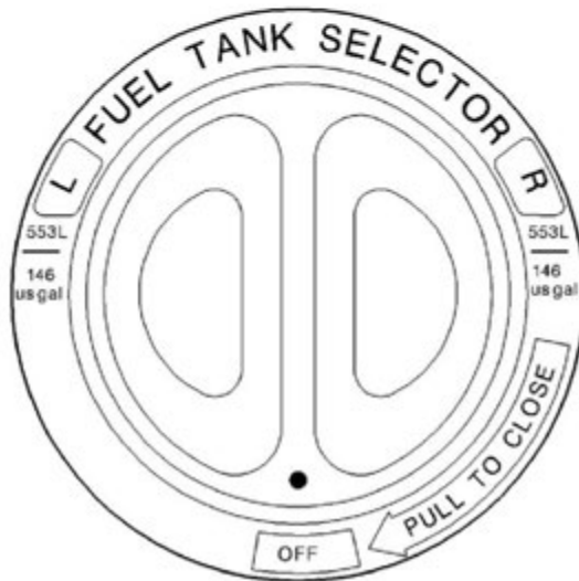
Figure 7.7.2 - Manual selector of fuel tanks
