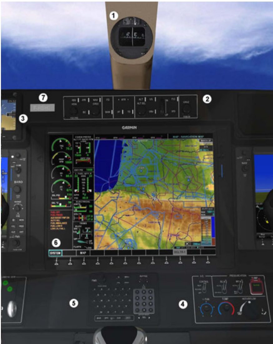
Figure 7.3.4A (2/2) - Central instrument panel (Typical arrangement) - Post-MOD70-0529-21
