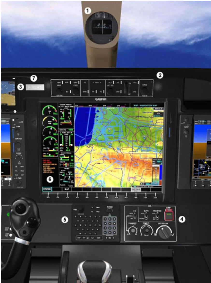
Figure 7.3.4 (2/2) - Central instrument panel (Typical arrangement) - Pre-MOD70-0529-21
