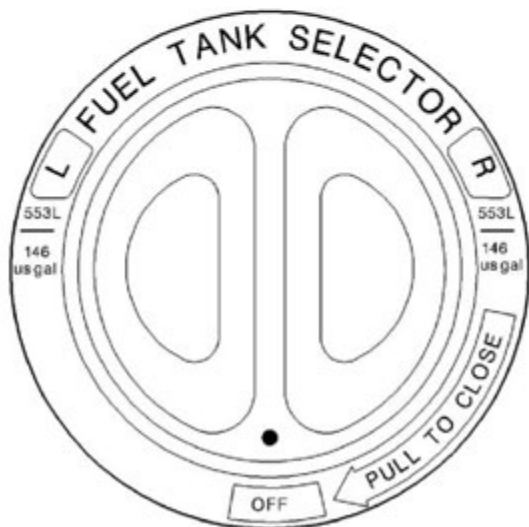
Figure 7.7.2 - Manual selector of fuel tanks
