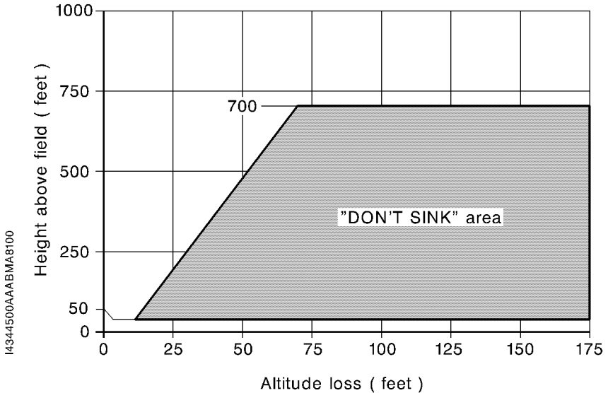
Figure 9.42.4 - "Don't sink" warning area
