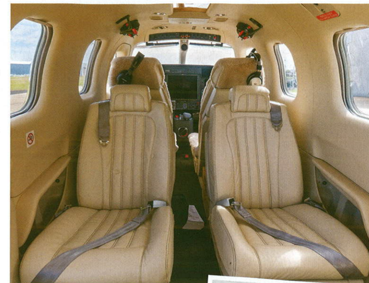
LEFT: The cabin is set-up in a four-seat club configuration with leather upholstered seats.
