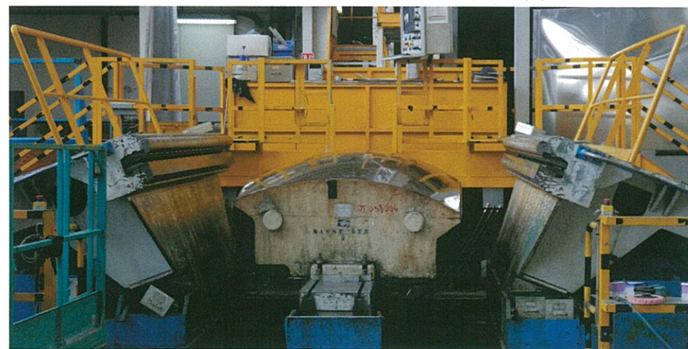
Aircraft panel (above) produced using the press below
