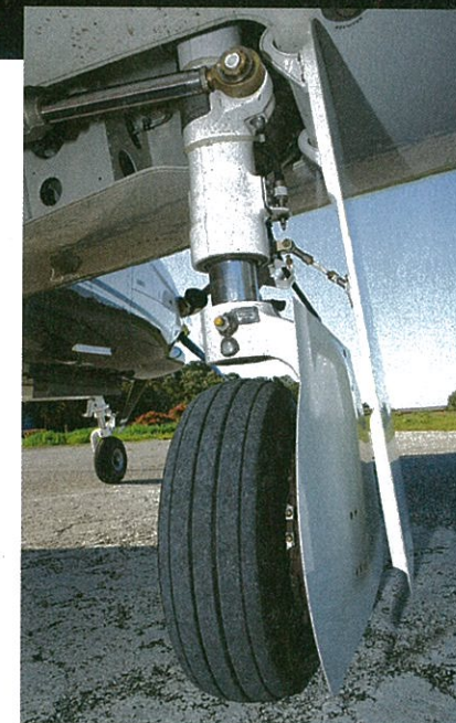
Landing lights have moved to the wingtip, and inner gear doors reduce drag on the TBM 900.
