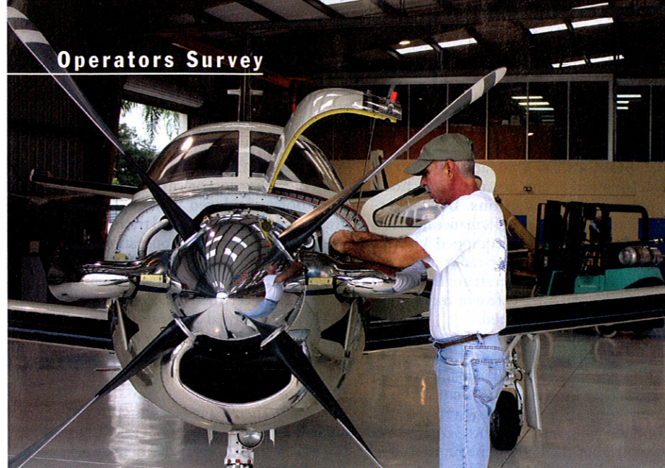
Operators say that the 850-shp PT6A-66D is powerful and reliable. But, the cost of overhaul at the 3,000 hour TBO is estimated to be $260,000 to $280,000.
