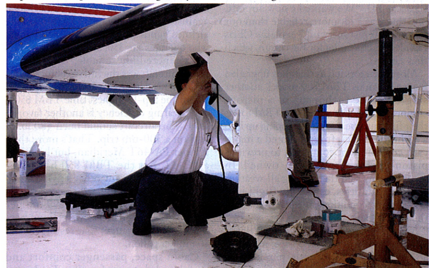
Daher-Socata worked with DRJ Technologies in Corona, Calif., to develop an overhaul program for the Messier-Dowty landing gear. Overhaul cost is one-third less than exchanging the components through Daher-Socata's own parts department. In addition, landing gear overhaul intervals have been extended to 5,000 cycles, thereby eliminating five- and seven-year calendar-based overhauls.
